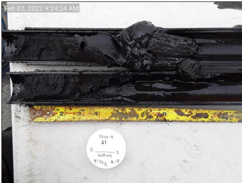
Figure 8. Organic river bottom sediment (typical) in Fox Point Reach. Sample S1 from depth 0 to 2 feet below ground surface (BGS) in boring FD22-11 (USACE 2022).
