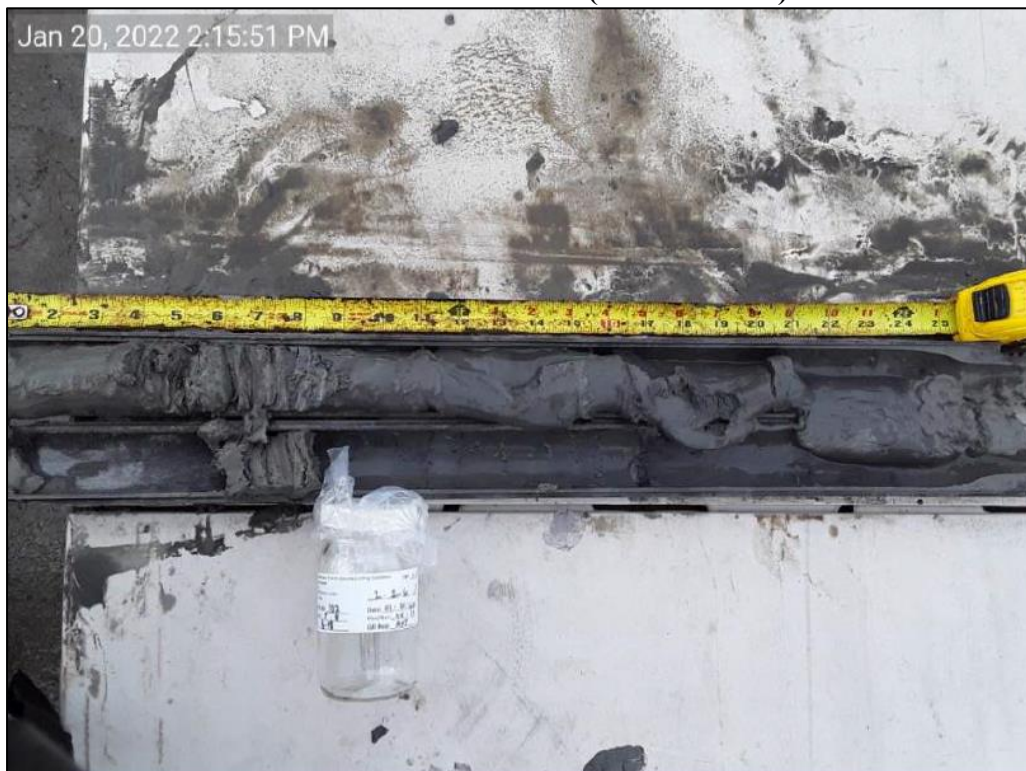
Figure 10. Inorganic river bottom sediment (typical) in Edgewood Shoals. Sample S8 from 16 to 18 feet BGS in boring FD22-02 (USACE 2022).
