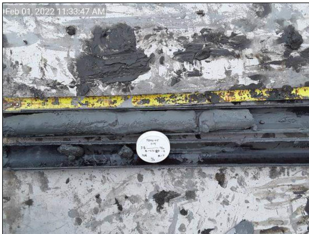
Figure 11. Glaciomarine outwash (typical) in Edgewood Shoals. Sample S14 from 38 to 40 feet BGS in boring FD22-05 (USACE 2022).
